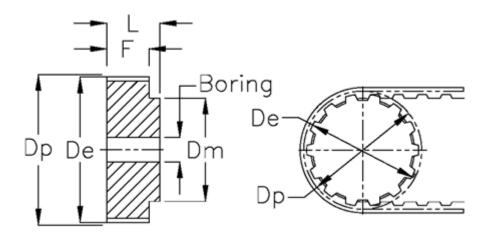
Type = T10Belt width = - 32 mm Weight = 3.004 = 189.1 De = 110 Dm = 191.1 Dp F = 37 L = 47 Pre-drilled = 16 Tooth number = 60
